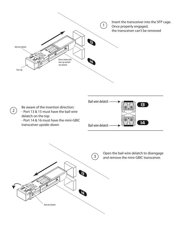
For any other model of mini-GBIC transceiver, please refer to the transceiver manual.
