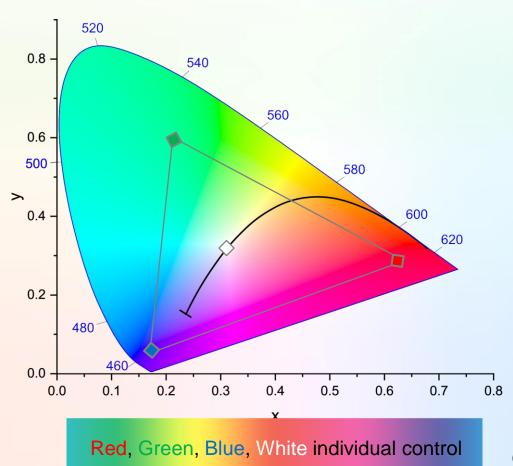
Red, Green, Blue and White control allows for deep saturated colours when needed
