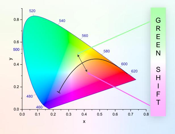
The HUE control allows for a +/- Green shift of 2 between 2800 and 6500K
