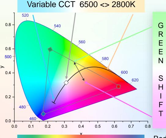
The HUE control allows for a +/- Green shift of 2 between 2800 and 6500K
