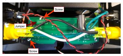
9. Included in the kit are two #4 Nylon 5/16" spacers. They must be positioned as shown in the photograph.
