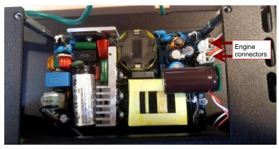
**6.** Remove the DMX connector (red and black wires), connected to the J7 pins on the PCB, to turn the assembly over and expose the internal components.
