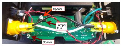
10. Install the wireless card on top of these spacers and into the jumper port as shown in the diagram. Use a #1 Phillips screwdriver to install the 2 - M3x20 screws included in the kit to secure the wireless card. If using a power driver, set torque to 5.5lb-in.
