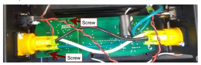
11. Turn the PCB Bracket Assembly right side up. Slide the back plate slightly up to expose the chassis. Insert the grommet attached to the antenna into the holes on the chassis. Ensure that the antenna does not come out of grommet. Slide the Back Plate at original position.
