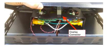
4. Remove the 4 x M3 screws from the PCB bracket assembly using a Philip's #1 screwdriver. If using a power driver, set torque to 5.5lb-in. Set screws aside. Remove the two washers that were underneath the 2 Knobs
