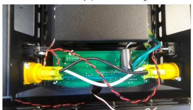
8. Remove the jumper from the PCB addressing card inside of the assembly. This will not be required after you install the wireless card. Remove the 2 x M3 screws from the PCB addressing card. These will not be required after you install the wireless card.
