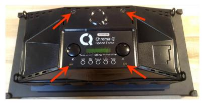
Carefully lift the back cover from the unit. The adjusting knobs will slide off with the cover. Remove the 5-pin overlay connector from the PCB board before completely removing the cover. Do not bend the pins. Set cover aside.
