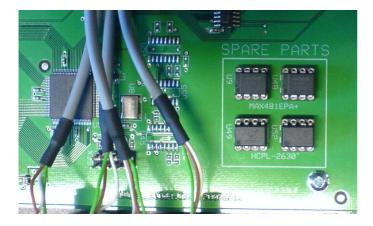
2 DMX transceivers and 2 optical couplers are provided to replace the ICs of a permanently broken DMX outlet.
